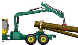
Log forwarding with quick-change clamping workbench
