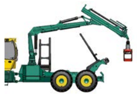
Rope forwarding possible Without reconfiguring the stanchion
