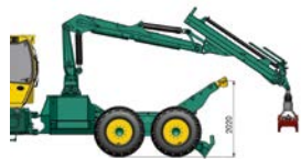
Height-adjustable pulleys Up to 2 m
