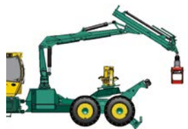
Rope forwarding possible without reconfiguring the clamping workbench
